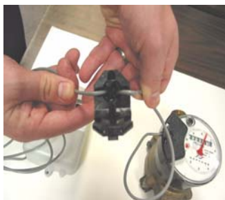
Figure 23 Gray Wires in Slots
