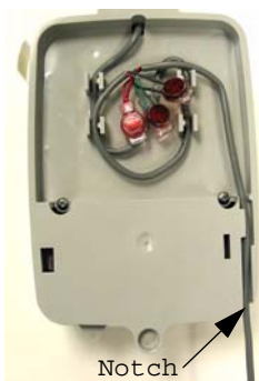
Figure 4 Cable Exit Notch.
