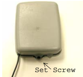
Figure 1 Wall MIU Main Housing
