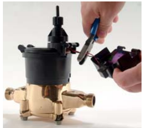
Figure 6 Cutting the Battery Wires
